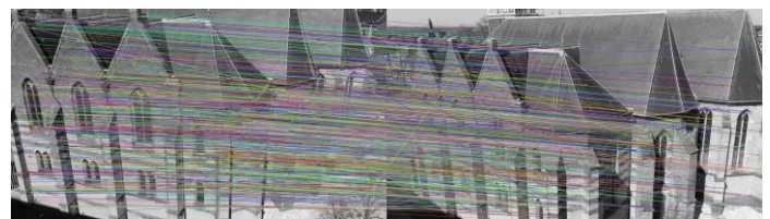
Fig.3 Feature matching of two frames we picked (Fig.1 and Fig.2) by brute-force SIFT matching.
